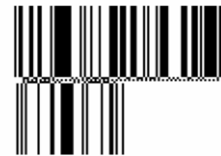
Figure 5.5.2.4.2 – 1: RSS Expanded Stacked Bar Code Symbol
