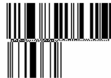
Figure 5.5.2.4.2 - 1: RSS Expanded Stacked Bar Code Symbol
