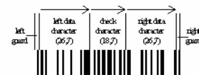
Figure 5.5.2.3 - 2: RSS Limited Bar Code Symbol Structure
