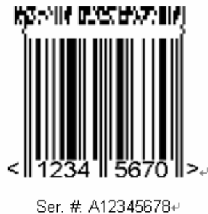
Figure 5.5.3.8 – 3: EAN-8 Symbol with a Three-Col
