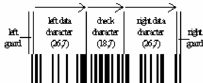
Figure 5.5.2.3 – 2: RSS Limited Bar Code Symbol Structure+
