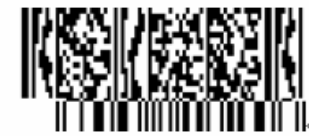
Figure 5.5.3.8 – 7: RSS Limited™ Symbol with a Three-Column CC-B
