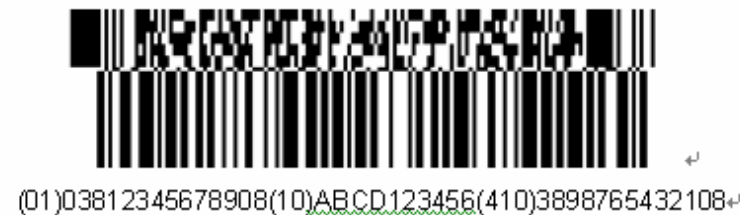
Figure 5.5.3.2 – 2: UCC/EAN-128 Composite Symbol with CC-C
