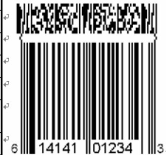
UPC-A Symbol with a Four-Column CC-B Component
