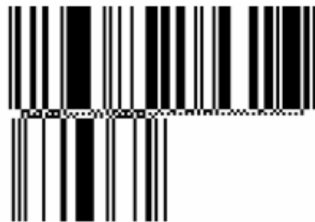
Figure 5.5.2.4.2 – 1: RSS Expanded Stacked Bar Code Symbol
