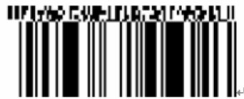
Figure 5.5.3.8 – 5: RSS-14™ Symbol with a Four-Column CC-A
