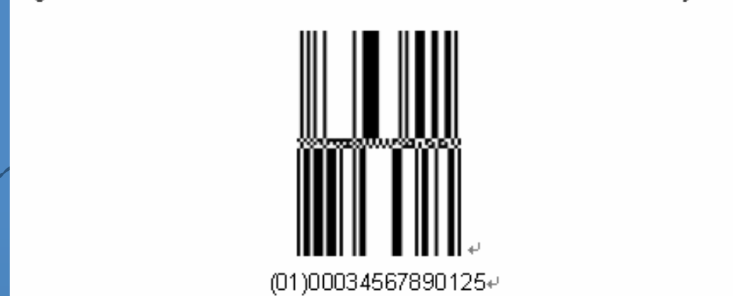
Figure 5.5.2.2.4 - 1: RSS-14 Stacked Omnidirectional Bar Code Symbol
