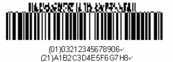
Figure 5.5.3.8 – 9: UCC/EAN-128 Symbol with a Four-Column CC-A
