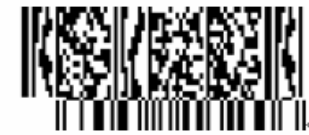
Figure 5.5.3.8 – 7: RSS Limited™ Symbol with a Three-Column CC-B
