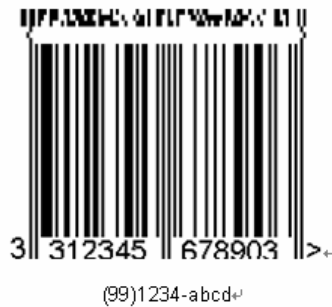
Figure 5.5.3.8 – 1: EAN-13 Symbol with a Four-Column CC-
