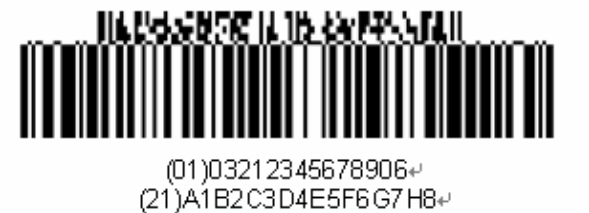
Figure 5.5.3.8 – 9: UCC/EAN-128 Symbol with a Four-Column CC-A
