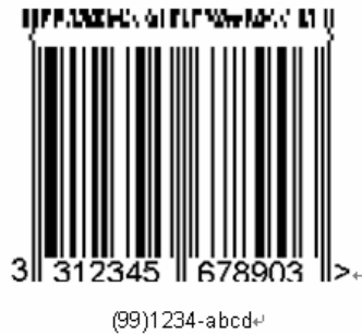
Figure 5.5.3.8 – 1: EAN-13 Symbol with a Four-Column CC-
