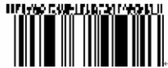
Figure 5.5.3.8 – 5: RSS-14™ Symbol with a Four-Column CC-A
