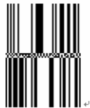
Figure 5.5.2.2.4 – 1: RSS-14 Stacked Omnidirectional Bar Code Symbol
