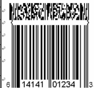
UPC-A Symbol with a Four-Column CC-B Component
