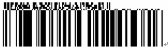
Figure 5.5.3.8 – 8: RSS Expanded™ Symbol with a Four-Column CC-A
