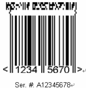
Figure 5.5.3.8 – 3: EAN-8 Symbol with a Three-Col
