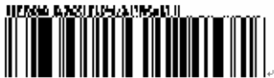
Figure 5.5.3.8 – 8: RSS Expanded™ Symbol with a Four-Column CC-A
