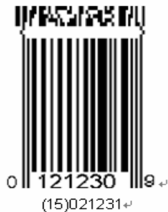
Figure 5.5.3.8 – 4: UPC-E Symbol with a Two-Column CC-A
