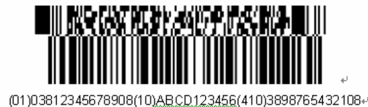
Figure 5.5.3.2 – 2: UCC/EAN-128 Composite Symbol with CC-C
