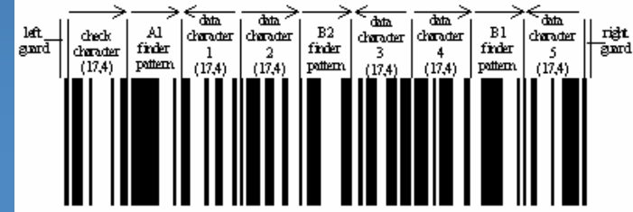
Figure 5.5.2.4 - 1: RSS Expanded Structure
